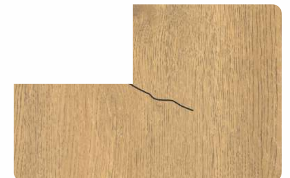
NO CLAIM WILL BE ENTERTAINED FOR CRACKING ARISING OUT OF GROOVE CURRRING OR L SHAPE.
